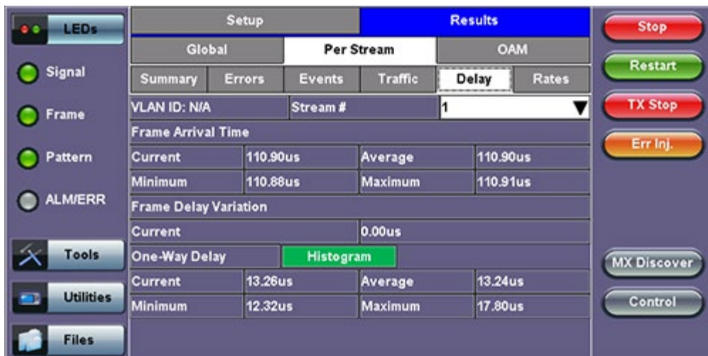
Throughput Results - Delay per Stream (One Way Delay)
