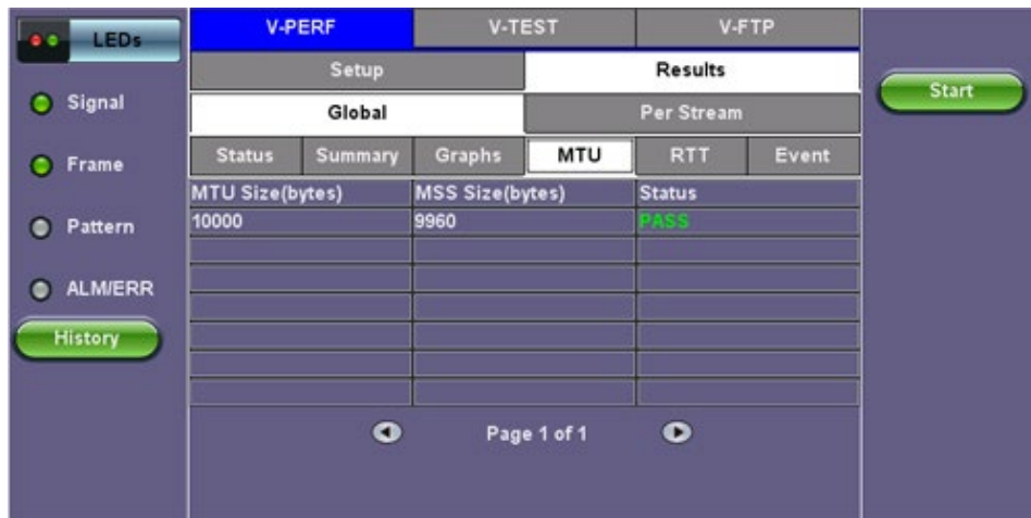
Test Set #2 - Client - Results - MTU
