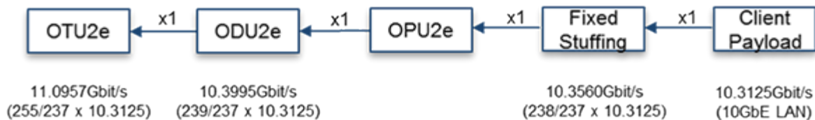
OTU2e (11.0957Gbps) bit rate support (with fixed stuffing)
