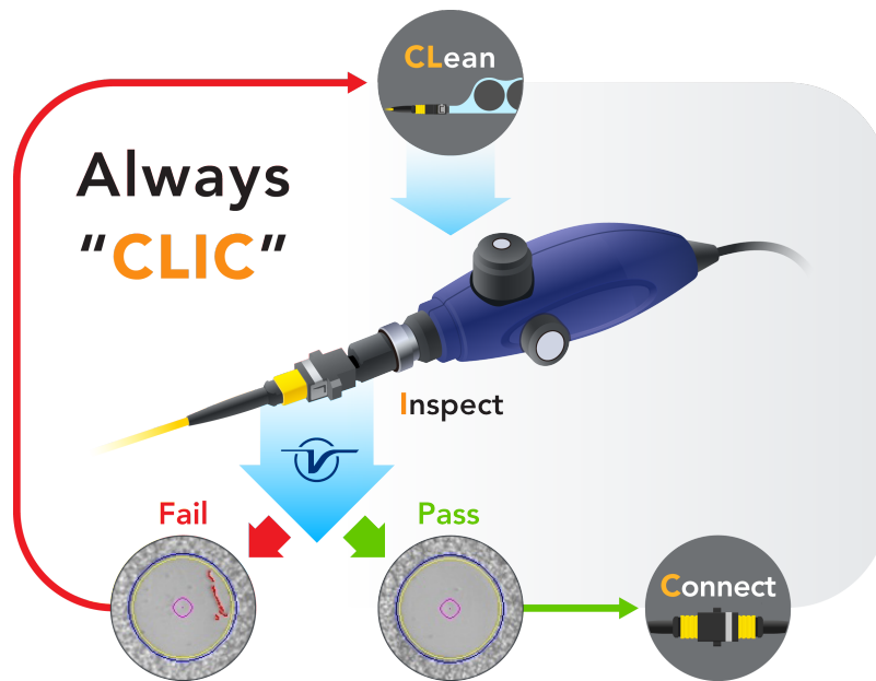
Best practices for inspection and cleaning prior to connecting an optical fiber
